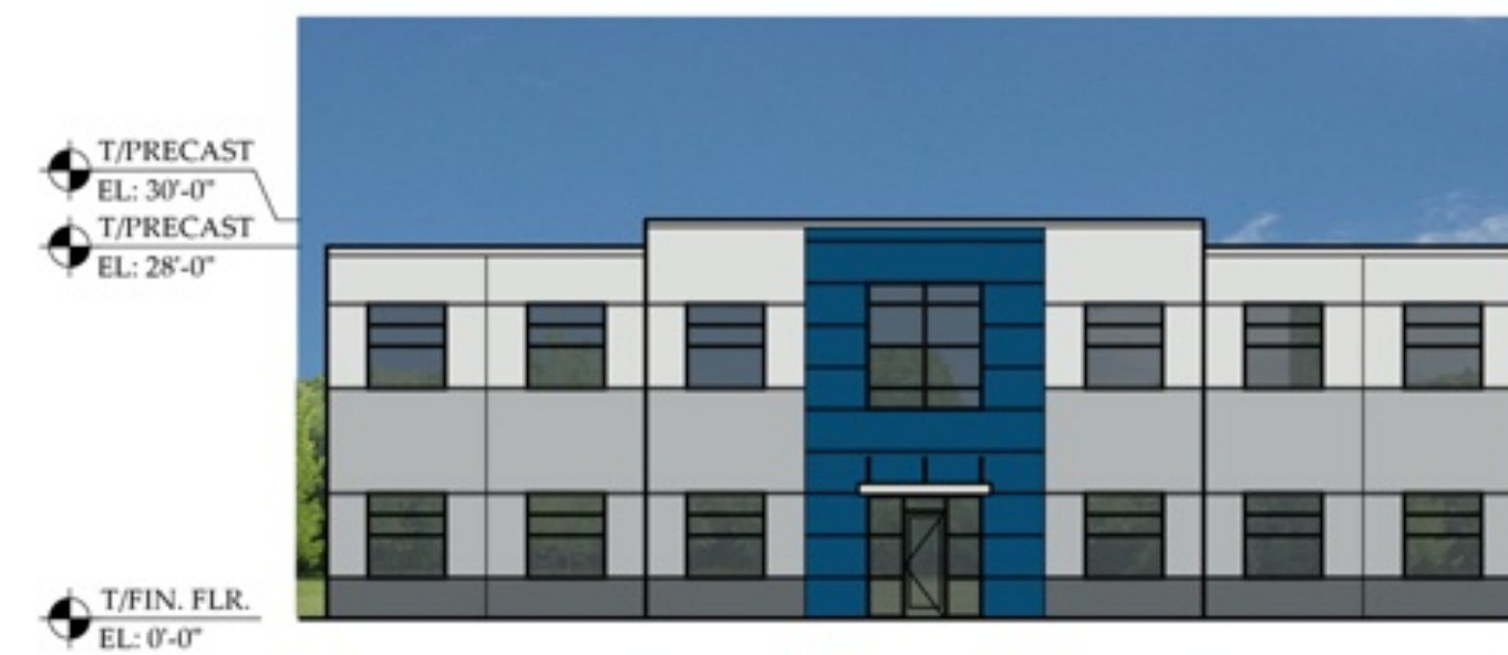
2 WEST ELEVATION SCALE: 1/16" = 1'
