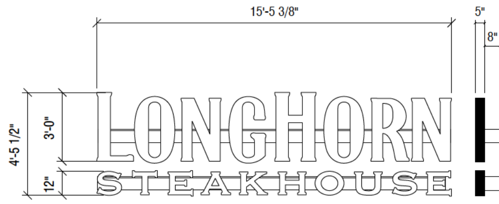
A 36" Channel Letters on Raceway (Internally Illuminated w/ LED) Utilized Square Footage: 68.9 SF Scale: 1/4"=1'
