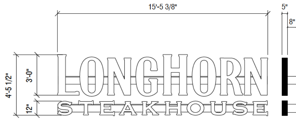
C 36" Channel Letters on Raceway (Internally Illuminated w/ LED) Utilized Square Footage: 68.9 SF Scale: 1/4" = 1'
